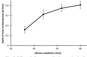
Fig. 7. Effect of vibrator amplitude onto depth of strain hardening layer
