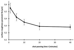
Fig. 3. Effect of shot peening time onto Ra surface roughness parameter
