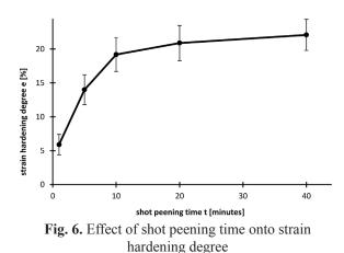
degree and such an increase was more visible in the scope of smaller values of shot peening parameters (Figures 5 and 6). The increase of shot peening time above 20 minutes caused only an insignificant increase of strain hardening degree.
