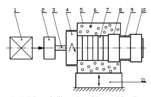
Fig. 1. Schematic illustration of the stand for vibratory and rotational shot peening: 1 – electric motor, 2 – reduction gear, 3 – flexible coupling, 4 – spindle,
